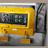
its and electrical function switches, rning horn are conveniently located on unted instrument panel. The instruments vidually replaceable "plug in" modular can be removed and replaced from the the instrument panel.
