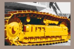
Long undercarriage provides unexcelled stability for fine grading and slope dozing. Seven (7) rollers distribute tractor weight evenly for excellent weight distribution.
