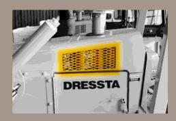
Insulated engine compartment utilizes hood side louvers and rear intake grill which provides high air flow for excellent cooling and low noise emissions.
