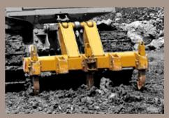
A versatile multi-shank ripper is a perfect choice for penetration tough materials and rip thoroughly to the depth of 429 mm (16.9").
